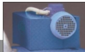
Electric filter shaking device standard on 3907/18.
