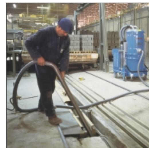
BLOCK MANUFACTURING: cleaning of ducts.
